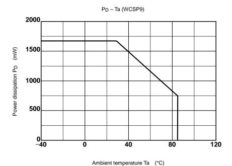
Please allow sufficient margin when designing a board pattern to fit the expected power dissipation. Also take into consideration the ambient temperature, input voltage, output current etc. and applying the appropriate derating for allowable power dissipation during operation.
