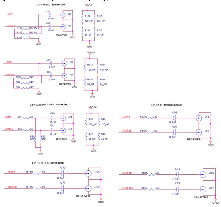
**Note**: For 2.5V and 3.3V HCSL termination, the C90 and C91 positions need to be assembled with 0  $\Omega$  resistors.
