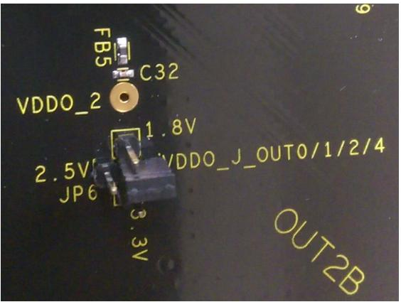
Note: Each output voltage can be individually selected. Use table 3 to select the jumper pin for its respective output:
