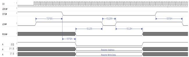
Note: It is recommended to keep CFG# asserted during the configuration write or read operation
