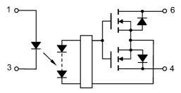
Fig. 5.1 Internal Circuit
