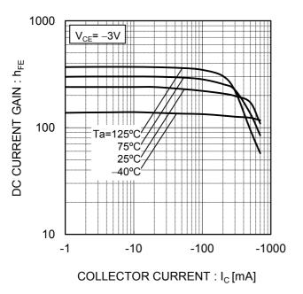
Fig.4 DC current gain vs. output current (II)
