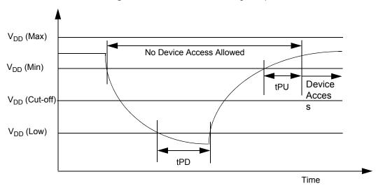
Figure 4.4 Power-Down and Voltage Drop
