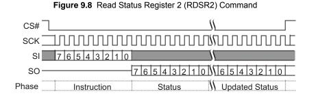
In Quad All mode, Status Register 2 may be read via the Read Any Register command, see Read Any Register (RDAR 65h) on page 91
