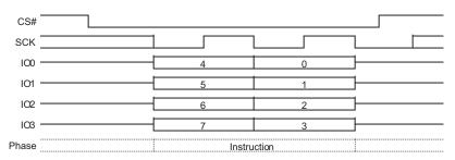
Figure 9.73 DPD Command Sequence QPI Mode
