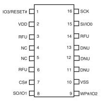
Figure 6.1 16-Lead SOIC Package, Top View
