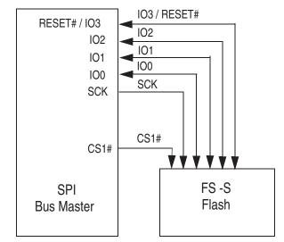
Figure 2.3 Bus Master and Memory Devices on the SPI Bus — Quad Bit Data Path
