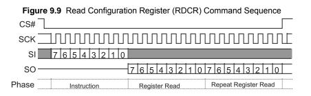
In Quad All mode, Configuration Register 1 may be read via the Read Any Register command, see Read Any Register (RDAR 65h) on page 91
