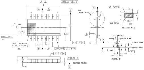
Figure 6.2 SOIC 16-Lead, 300-mil Body Width (SO3016)
