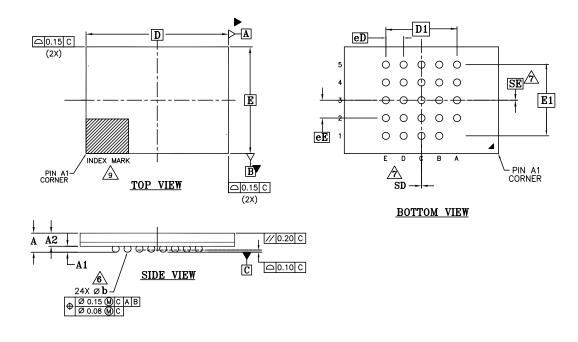
Figure 6.6 Ball Grid Array 24-Ball 6x8 mm (FAB024)
