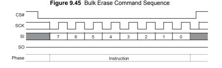
This command is also supported in QPI mode. In Quad All mode the instruction is shifted in on IO0-IO3, two clock cycles per byte.
