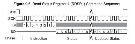
This command is also supported in QPI mode. In Quad All mode the instruction is shifted in on IO0-IO3 and the returning data is shifted out on IO0-IO3, two clock cycles per byte.
