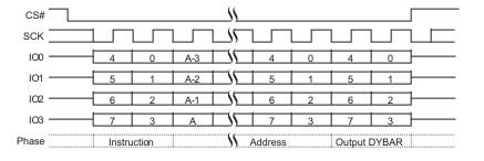
Figure 9.57 DYBRD QPI Mode Command Sequence
