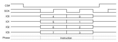
Figure 9.75 RES Command Sequence QPI Mode
