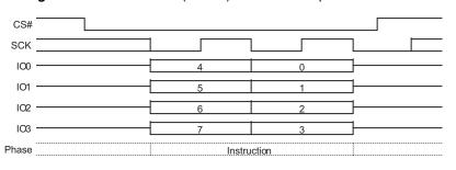
Figure 9.14 Write Enable (WREN) Command Sequence QPI Mode
