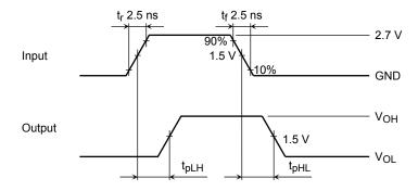
Figure 2 t<sub>pLH</sub>, t<sub>pHL</sub>
