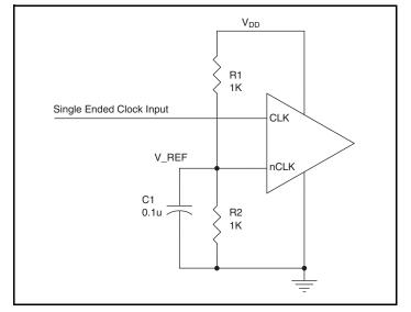
Figure 2. Single-Ended Signal Driving Differential Input
