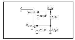
Figure 1. Power Supply Filtering
