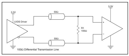
Figure 4. Typical LVDS Driver Termination
