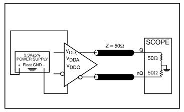
3.3V LVDS Output Load AC Test Circuit
