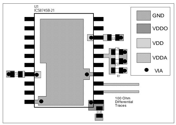
Figure 5B. PCB Board Layout for 8745B-21
