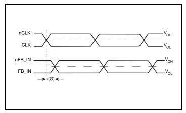
Phase Jitter and Static Phase Offset
