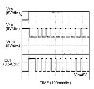
Figure 33. Over-current response Enable to short circuit
