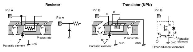
Figure 41. Example of monolithic IC structure
