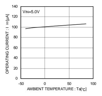
Figure 5. Operating current EN,/EN enable
