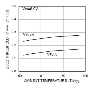
Figure 16. UVLO threshold
