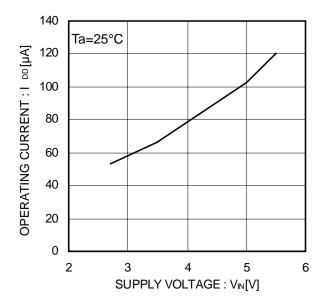
Figure 4. Operating current EN,/EN enable
