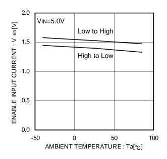
Figure 9. EN,/EN input voltage
