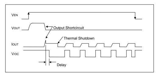
Figure 38. Over-current detection, Thermal shutdown timing (BD2226G)
