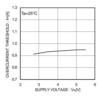
Figure 12. Over-current threshold
