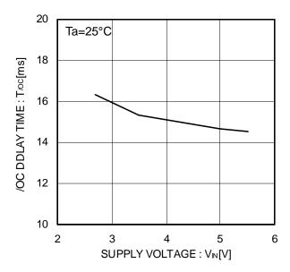
Figure 26. /OC delay time
