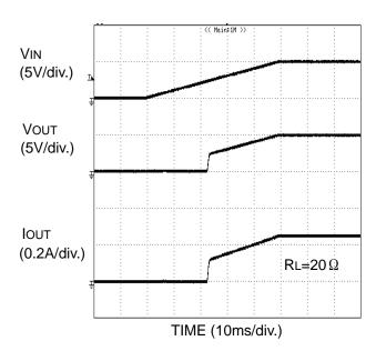
Figure 35. UVLO response Increasing VIN
