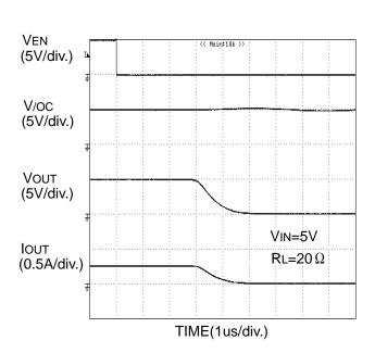
Figure 29. Output fall characteristic
