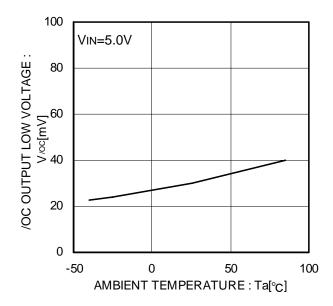
Figure 15. /OC output low voltage
