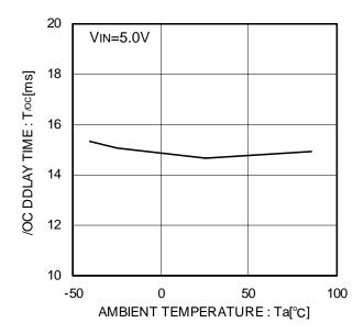
Figure 27. /OC delay time
