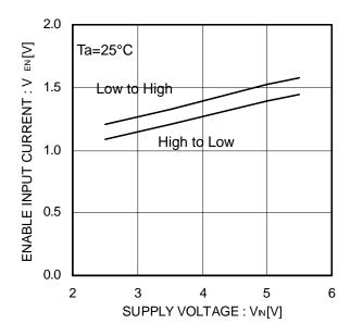
Figure 8. EN,/EN input voltage
