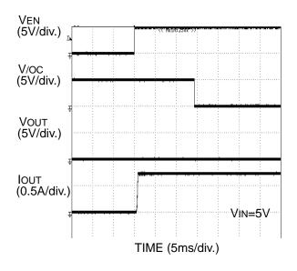
Figure 32. Over-current response Enable to short circuit
