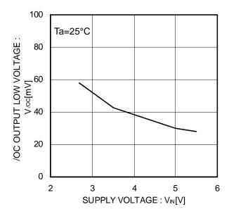
Figure 14. /OC output low voltage
