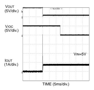
Figure 34. Over-current response  $1\Omega$  load to enabled device
