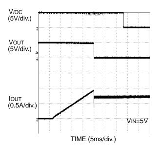
Figure 31. Over-current response ramped load
