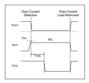
Figure 37. Over-current detection
