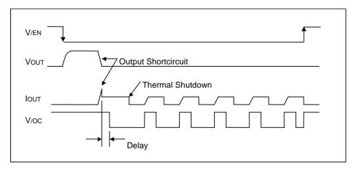
Figure 39. Over-current detection, Thermal shutdown timing (BD2227G)
